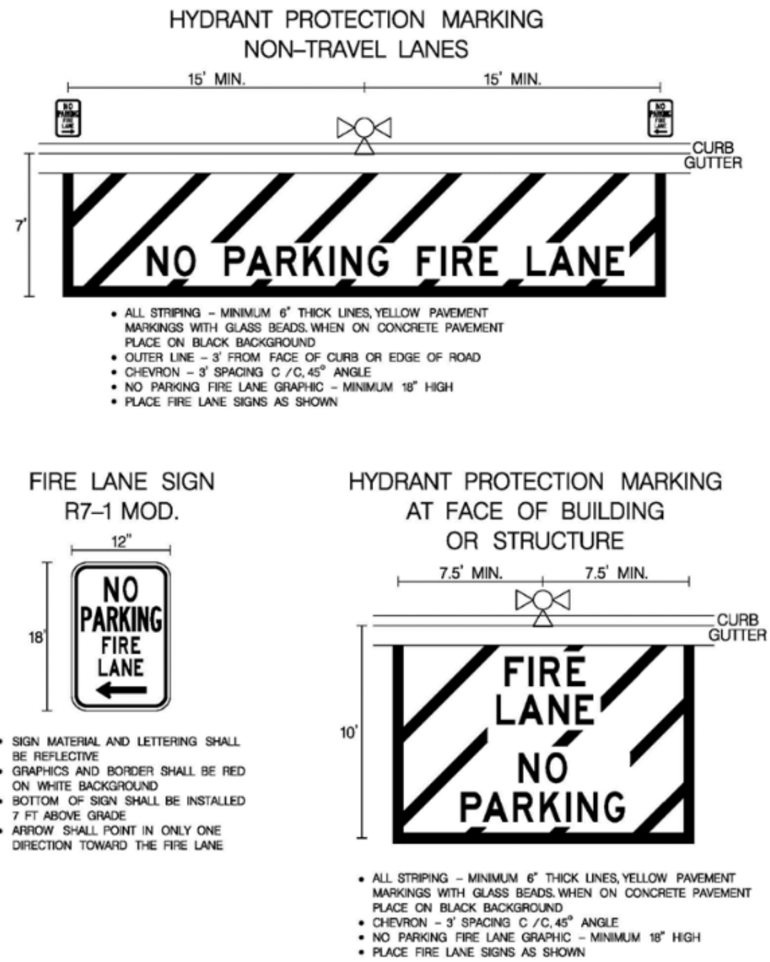
Figure 3.1.16.4-1 – Fire Lane Markings at Hydrants
